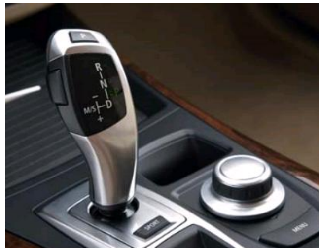
BMW electronic gear selector and Steptronic
